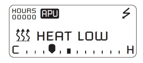
Press again to switch between high and low heat to heat the truck bunk more or less quickly. In "**HEAT HIGH**" mode, the power outlet is disabled and the display indicates . The heat will turn off when the desired temperature is reached.
